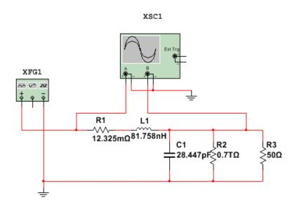
The R, L, and C components can be found by right clicking and clicking "Place component." Then on the left side, under group, select the "Basic." group. Resistors, capacitors and inductors can be found under the family section on the left hand side. Since we will be changing the values of each element, it doesn't matter which value you initially choose. Additionally, the ground component can be found under the "Sources" group and the "POWER\_SOURCES" family with the title "GROUND."
